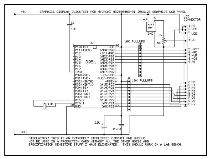
I used an Atmel 89C52 which holds up to 8-Kbytes of code, but the demonstration code is only 160 bytes. The crystal is a 12 MHz parallel resonant crystal, but use whatever suits you. Technically, you shouldn't require the pullups on port 2 driving the LCD data bus, but I found that the internal microcontroller pullups are too weak and the bus doesn't rise from "0" to "1" quickly enough when doing successive writes. Also, you'd normally put 22-pF caps on each leg of the crystal to
