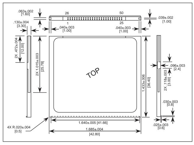
Figure 2-1. CompactFlash Memory Card Dimensions
