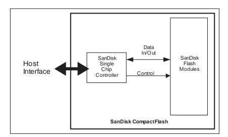
Figure 1-1. CompactFlash Memory Card Block Diagram
