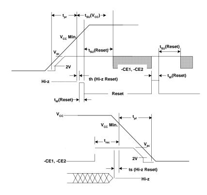
Figure 3-1. Power-Up/Power-Down Timing for Systems Supporting RESET
