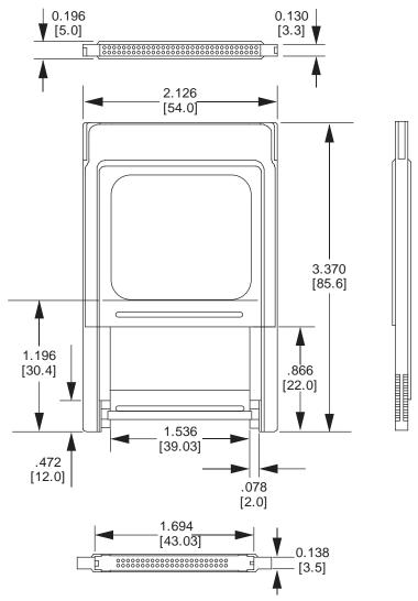
Figure 2-2 CompactFlash Memory Card Adapter Dimensions
