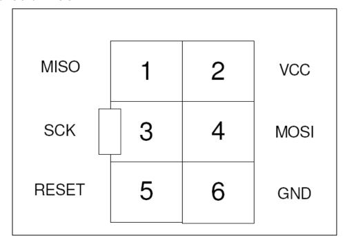
Kanda supply a 10-way to 6-way adapter, which plugs into the end of the programmer lead, for use with targets with this connector. Please see
