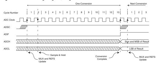
Figure 45. ADC Timing Diagram, Auto Triggered Conversion
