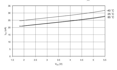
Figure 124. ADC Current vs. V<sub>CC</sub>
