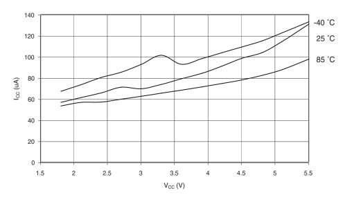
Figure 126. Programming Current vs.  $V_{CC}$
