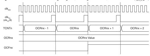
Figure 36 shows the setting of OCF0A and the clearing of TCNT0 in CTC mode and fast PWM mode where OCR0A is TOP.
