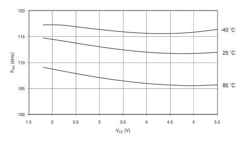
Figure 122. 128 kHz Watchdog Oscillator Frequency vs. Temperature
