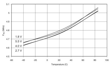
Figure 119. Calibrated 4.8 MHz RC Oscillator Frequency vs.  $V_{\rm CC}$
