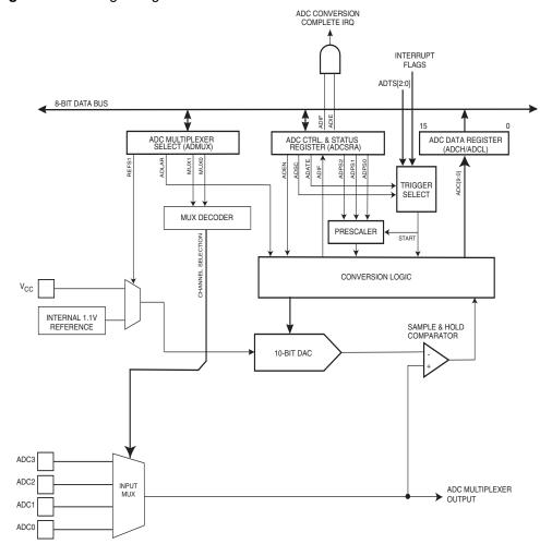
Figure 40. Analog to Digital Converter Block Schematic
