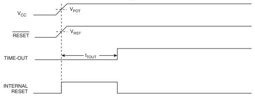
Figure 15. MCU Start-up, RESET Extended Externally
