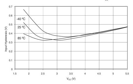
Figure 106. Reset Input Threshold Voltage vs.  $V_{CC}$  (VIH, Reset Pin Read as '1')
