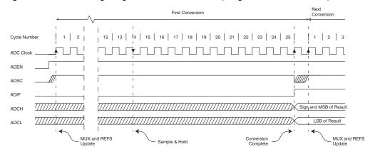
Figure 44. ADC Timing Diagram, Single Conversion
