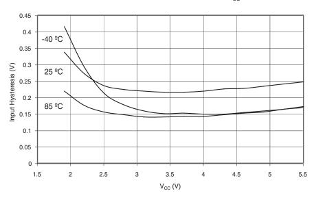
**Figure 103.** Reset Pin as I/O - Input Threshold Voltage vs.  $V_{\text{CC}}$  (VIH, Reset Pin Read as '1')
