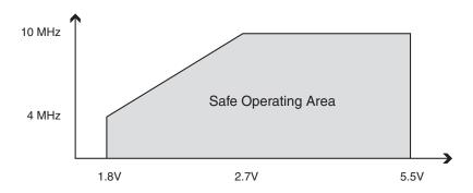
Figure 63. Maximum Frequency vs. V<sub>CC</sub>, ATtiny13
