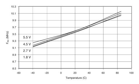
Figure 116. Calibrated 9.6 MHz RC Oscillator Frequency vs.  $V_{\rm CC}$
