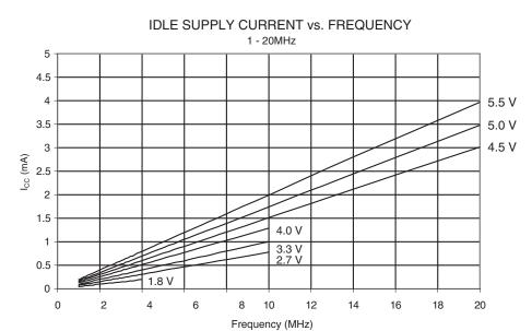
Figure 71. Idle Supply Current vs. Frequency (1 - 20 MHz)
