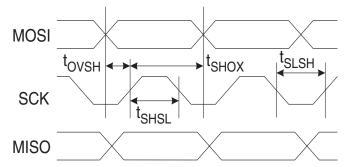
**Table 51.** Serial Programming Characteristics,  $T_A = -40^{\circ}C$  to 85°C,  $V_{CC} = 1.8 - 5.5V$  (Unless Otherwise Noted)
