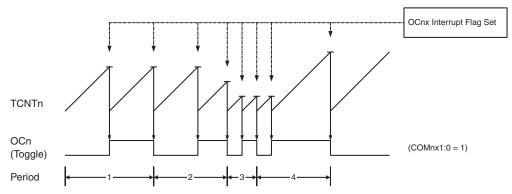
An interrupt can be generated each time the counter value reaches the TOP value by using the OCF0A Flag. If the interrupt is enabled, the interrupt handler routine can be used for updating the TOP value. However, changing TOP to a value close to BOTTOM when the counter is running with none or a low prescaler value must be done with care since the CTC mode does not have the double buffering feature. If the new value written
