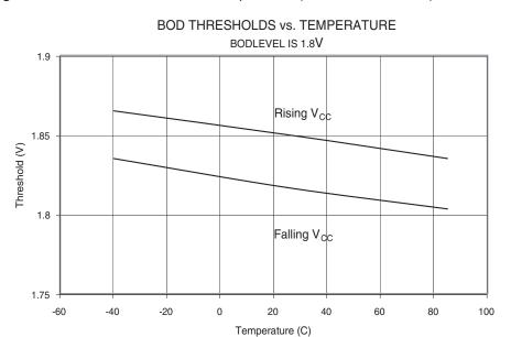
Figure 111. BOD Thresholds vs. Temperature (BODLEVEL is 1.8V)
