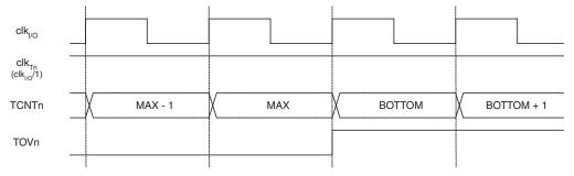
Figure 34 shows the same timing data, but with the prescaler enabled.
