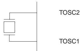
Figure 8-3. Crystal Oscillator Connections
