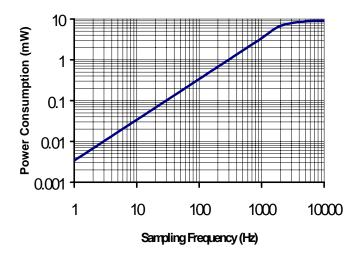
Figure 2. ADXL150 Average Power Consumption vs. Power Cycling Frequency
