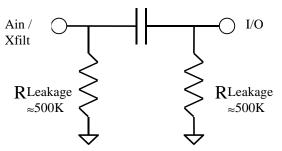
Figure 6. Model of Microcontroller Ports When in Tri-State Mode
