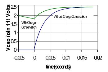
342mg) versus the steady state output after 10ms. To get to within 92mg of steady state output without charge conservation we would have had to wait 14.1ms After turn-on. Resulting in an average current consumption of:
