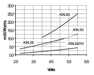
Figure 1. Power consumption vs Supply Voltage for Several Accelerometers If the entire system is ratiometric (i.e. the A to D reference voltage is proportional to Vdd) this reduction of sensitivity is not a problem. A potentially more serious problem is that the accelerometer's noise performance is generally degraded as the supply voltage is reduced. This cannot be mitigated by using a ratiometric system, and must be kept in mind during system design.
