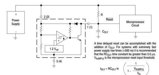
Figure 8. Low Voltage Microprocessor Reset
