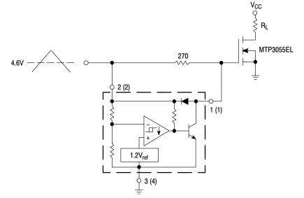
Overheating of the logic level power MOSFET due to insufficient gate voltage can be prevented with the above circuit. When the input signal is below the 4.6 V threshold of the MC34064, its output grounds the gate of the  $L^2$  MOSFET.
