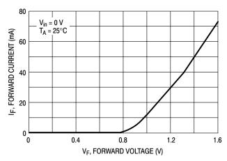
Figure 7. Clamp Diode Forward Current versus Voltage
