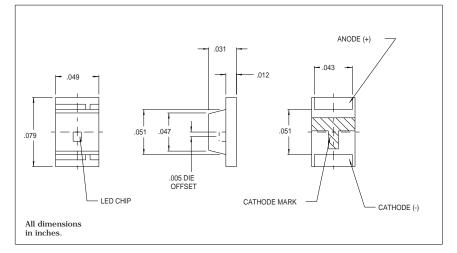
•Premium brightness in miniature chip-type LED assemblies. •Integral reflection cup maximizes output •Ideally suited for applications such as telecommunications, data processing peripherals and networking units as
