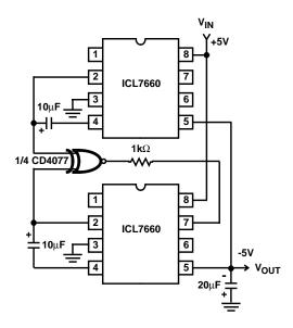
FIGURE 14. SYNCHRONIZING TWO ICL7660S
