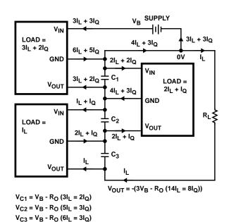
FIGURE 17. CURRENT FLOW FOR CASCADED DEVICES
