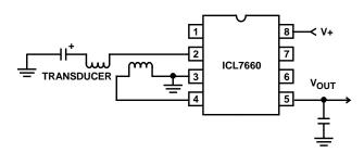
FIGURE 24. TRANSDUCER DRIVER AND DETECTOR
