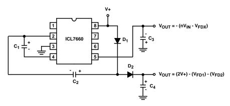
FIGURE 19. COMBINED NEGATIVE CONVERTER AND POSITIVE MULTIPLIER
