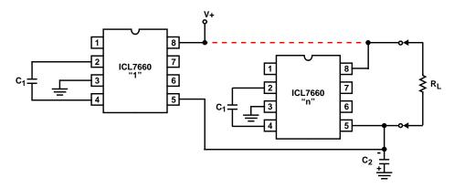
FIGURE 13. PARALLELING DEVICES
