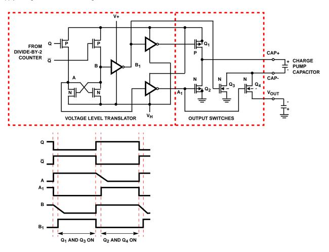
FIGURE 4. THE ICL7660S OUTPUT SWITCHES AND VOLTAGE LEVEL TRANSLATOR CIRCUIT
