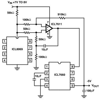
FIGURE 22. REGULATED OUTPUT INVERTER
