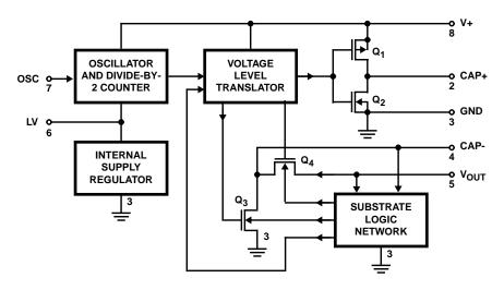
FIGURE 2. FUNCTIONAL DIAGRAM OF COMPLETE CHIP
