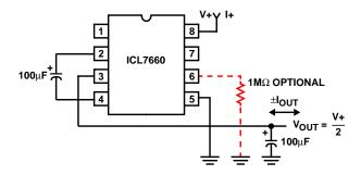
FIGURE 20. EFFICIENT SUPPLY SPLITTING
