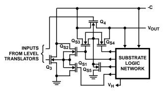
FIGURE 5. THE SUBSTRATE LOGIC NETWORK
