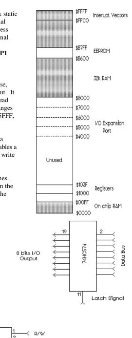
For example, if you connect up pin 11 *latch enable* of a 74HC574 to pin 9 of the 74HC138 and then a program write of \$FF to address \$7000, will make all output pins on 74HC574 high. A write of \$00 to address \$7000 will make all output pins would go low.
