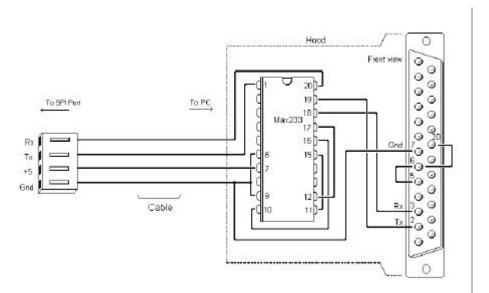
The 9 pin serial connector on the BOTBoard 2 is a DB9F and is designed to connect to a PC serial port with 9 pin straight through extension cable. The output of the DB9F is true RS232 levels because of the MAX232 level converter. If you need TTL level serial signals, use the SCI port.
