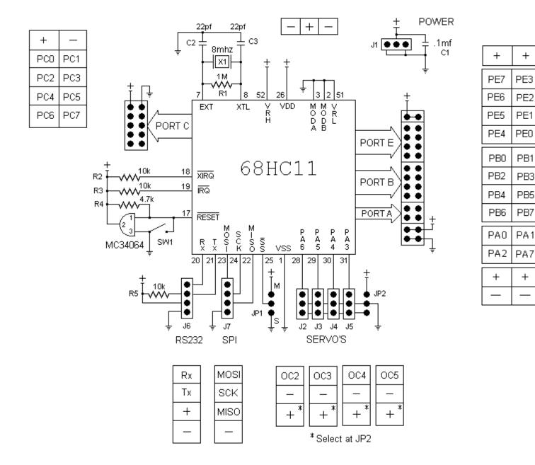
**Note:** I have had good success replacing the MC34064 with a .1mf capacitor between pins one and three, and changing R4 to a 10k resistor. Please refer to Motorola documentation on reset and low voltage reset.
