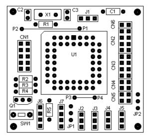
1. The first components mounted to the BOTBoard is the two jumpers, P1-P2 and P3-P4. Simply strip two wires, to the appropriate length and solder into position.
