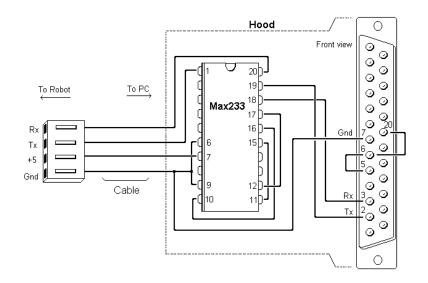
**The MAX232** is a 16 pin IC that uses four 1.0Mf capacitors to boost the chips voltage. This chip is very inexpensive and is readily available.
