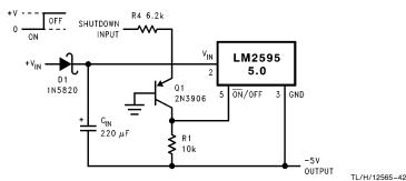
FIGURE 27. Inverting Regulator Ground Referenced Shutdown
