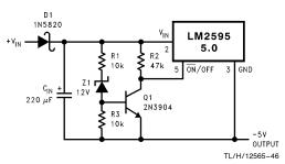
This circuit has an ON/OFF threshold of approximately 13V.
