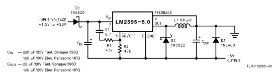
FIGURE 25. Inverting -5V Regulator with Delayed Startup
