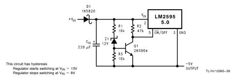
FIGURE 24. Undervoltage Lockout with Hysteresis for Inverting Regulator
