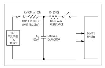
Figure 7a. IEC1000-4-2 ESD Test Model
