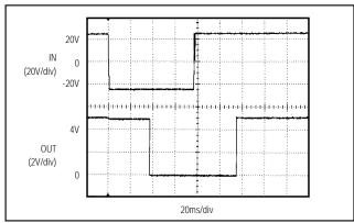
Figure 3. Switch Input ±25V Fault Tolerance
