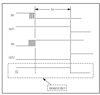
Figure 2. Input Characteristics
