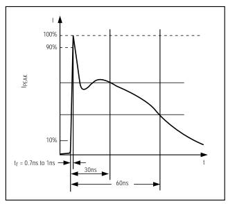
Figure 7b. IEC1000-4-2 ESD Generator Current Waveform
