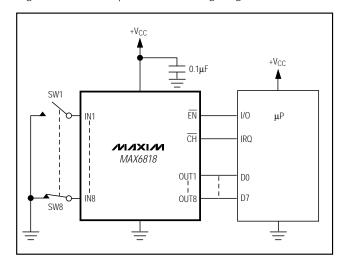
Figure 5. MAX6818 Typical µP Interfacing Circuit
