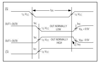
Figure 4. MAX6818 µP-Interface Timing Diagram
