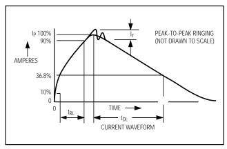
Figure 6b. Human Body Current Waveform
