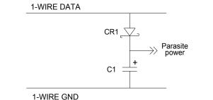
Using a Schottky diode and capacitor to supply local power on the 1-Wire net.
