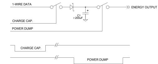
A parasite-powered 1-Wire remote high-energy source concept.
