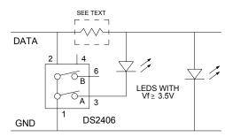
Using the power available between 3.5V and 5V directly and under bus master control.
