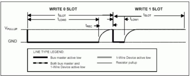
Figure 2. 1-Wire write time slots.
