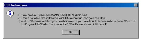
From the USB Instruction screen you get to the 1-Wire Net Port Selection screen, on which you must specify which of the ports with a 1-Wire adapter connected is to be defined as the **default 1-Wire Net port**. It is possible to have more than one port adapter plugged in at a time. However, only one of them can be selected as the default.
