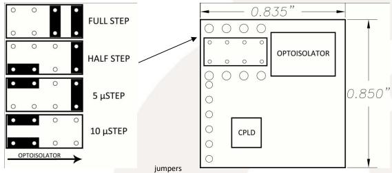
have been located they may be set according to the diagram below. Please note that the four pins closest to the optoisolator are unconnected and can be used as jumper storage. It is recommended that needle nose pliers or tweezers be used to adjust the jumper settings. The power to the G213V must be turned off before any adjustment is to be made on the step pulse multiplier.
