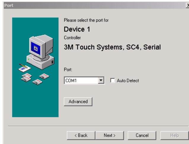
Figure 7: Selecting COM port for Windows driver (Do not select Auto Detect)
