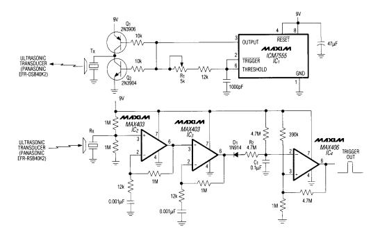
Figure 1. Comprising an independent transmitter and receiver, this battery-powered, ultrasonic proximity detector features two 40kHz piezo-ceramic transducers.
