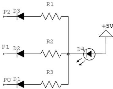
$300\text{ohms} \leq R_i \leq 400\text{ohms}$ . The 74HC374 can sink over 20mA per pin. By using software control of the LED level, a range of 0.5 to 44 inches (a little over a meter) can be realized. The algorithm for achieving a meter range requires the software to start at the highest level  $P2=P1=P0=GND$  and decrease the level if the response is saturated at 2.5V. To achieve optimum accuracy, one should select the resistor range that drives the analog signal as close to 2.0V as possible.
