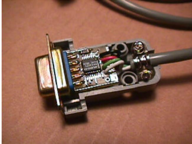
The RS232/DB9 is designed to convert TTL level signals into RS232 level signals. This cable allows you to connect a TTL level device, such as the serial port on a Micro-controller, to the serial port of a personal computer. The conversion circuit is housed inside the DB9 connector shell. Power is supplied from the Micro-controller board.
