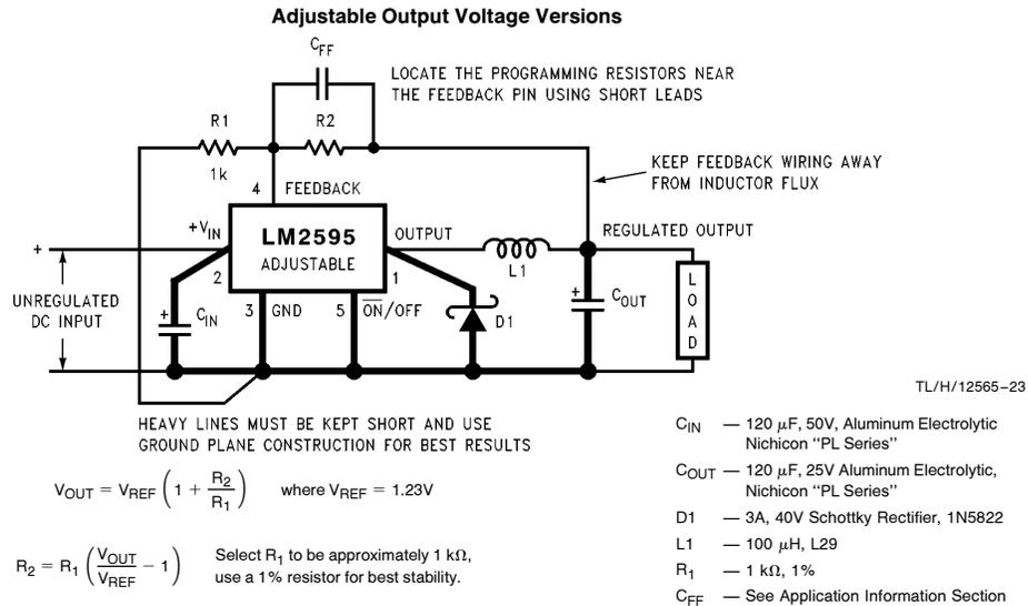
$$V_{OUT} = V_{REF} \left( 1 + \frac{R_2}{R_1} \right) \quad \text{where } V_{REF} = 1.23\text{V}$$
