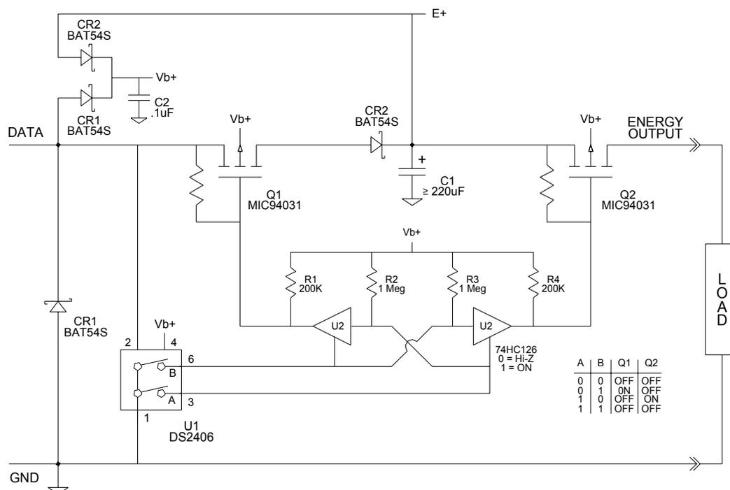
An isolated remote energy source based on the DS2406 addressable switch.
