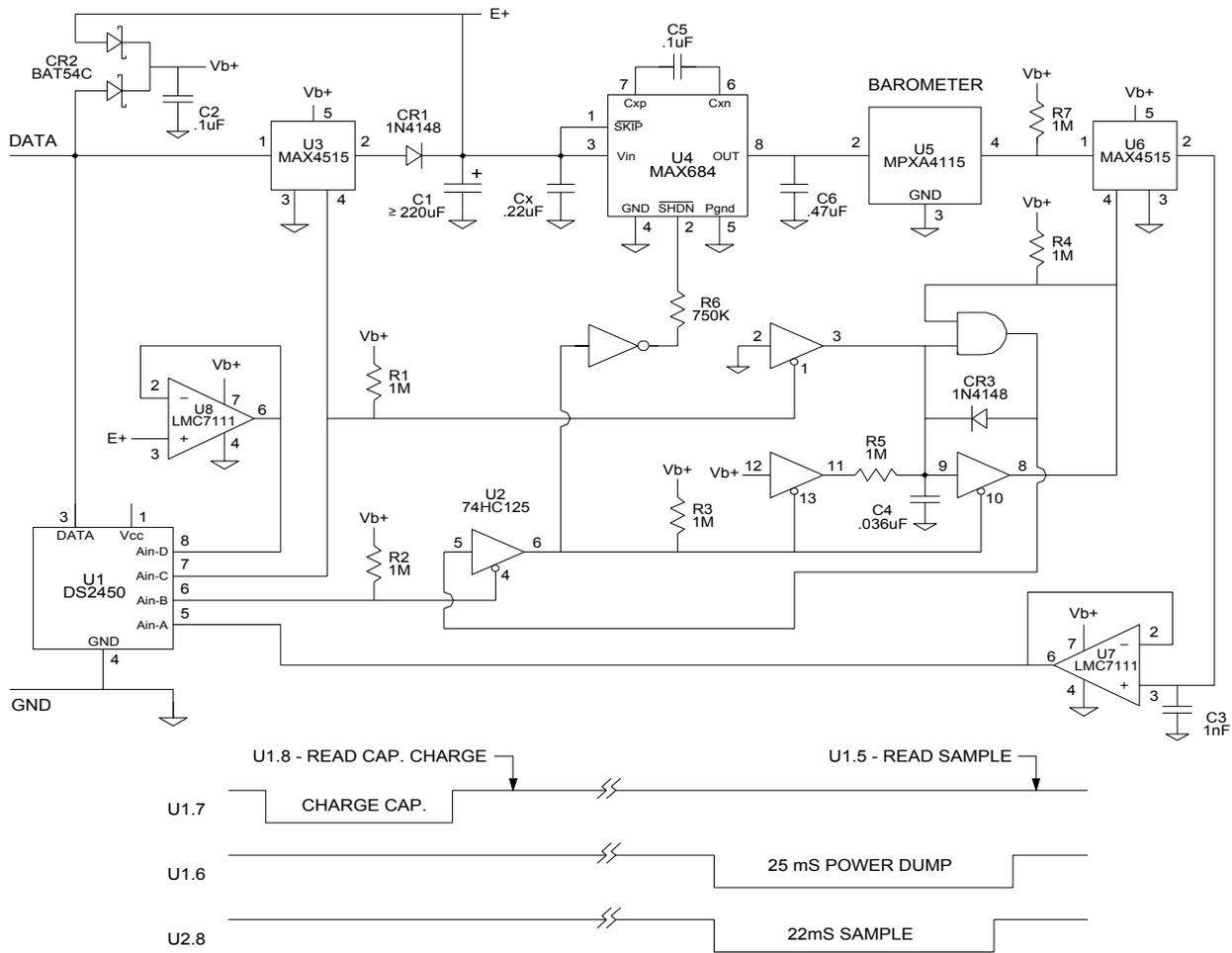
A 1-Wire barometer powered off the bus by an isolated and regulated energy source.
