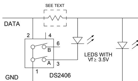
Using the power available between 3.5V and 5V directly and under bus master control.
