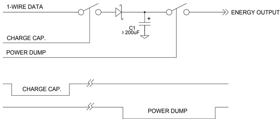
A parasite-powered 1-Wire remote high-energy source concept.
