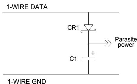
Using a Schottky diode and capacitor to supply local power on the 1-Wire net.
