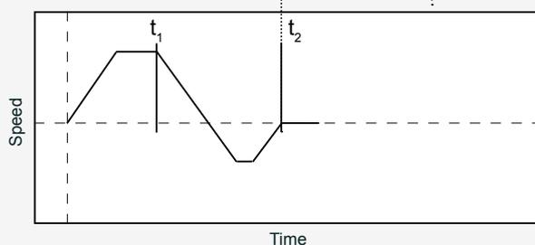
$t_1$  : Second command position given, servo drive immediately targets to second position
